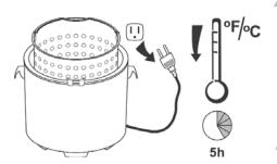
▲ DANGER: Disconnect electric cord from outlet, before cleaning, servicing and/or removing heating element. Electrical shock can result in personal injury or death.
